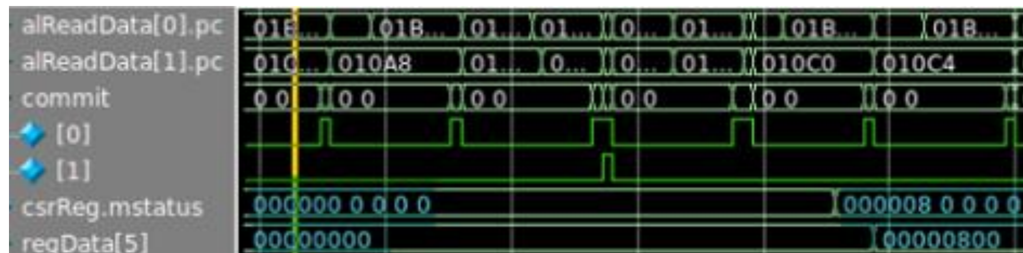
Figure 6: Simulation waveform showing the processor switching privilege contexts from Machine to Supervisor.
